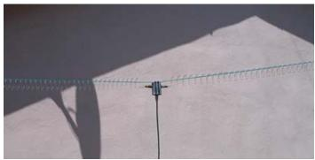
A longer range view showing a nearly 40-meter configuration. In this shot the coils are stretched out about 8 feet in either direction and held in place with alligator clips attached to the messenger line. In the final version there will a lighter cord attached to the end of each coil so the length can be adjusted at will.
