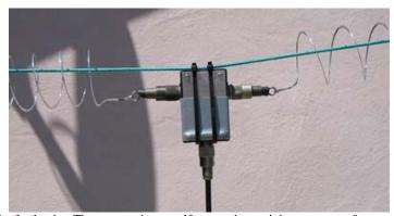
Here's a close-up of the feed point. The antenna is not self supporting so it is strung on a "messenger line" which is just a length of nylon cord stretched tight between two supports.
