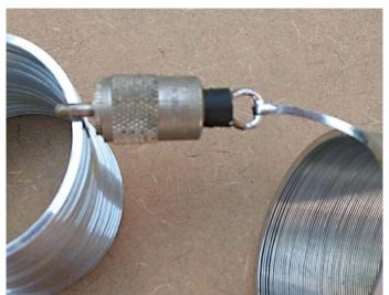
This photo shows the detail of connecting the Slinky to the loop of wire. Cut the end off the Slinky at the clip and bend a look in it with a pair of thin nosed pliers. Hook it into the loop of wire and crimp it down with the pliers. Apply lots of solder and you're all set.
